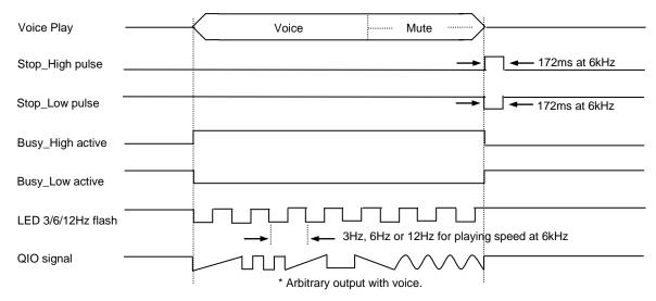
LED dynamic 1/2: When the voice amplitude is higher than 1/2 level, LED will be ON, i.e. output signal is low.
