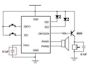
Note: At high voltage of 4.5V or higher voltage, VREG may be connected to GND with a 0.1uF cap for less power noise. At 3V, VREG doesn't need to connect any capacitor and can be kept this pad floating to save a capacitor.
